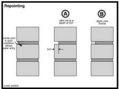
The masonry mortar joints at the front of the house show signs of deterioration and should be repointed (1B.07).
